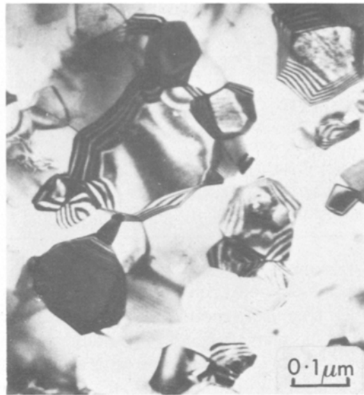
Figure 2 A bright-field transmission electron micrograph of CVD TiC in the "interfacial carbide" layer.
